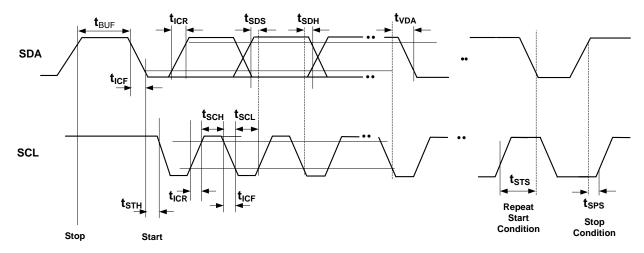
Figure 2. I<sup>2</sup>C Timing
