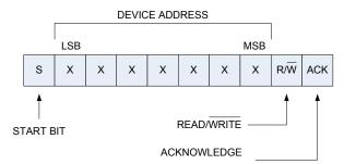
Figure 37. I<sup>2</sup>C Device Addressing
