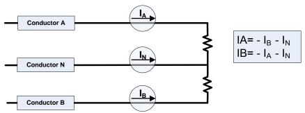
Figure 13. Current Input Configuration
