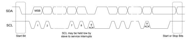
Figure 36. I<sup>2</sup>C Bus Characteristics
