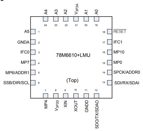
Figure 3. QFN Package Pinout
