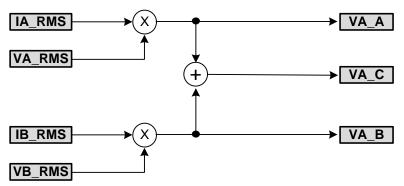
Figure 23. Apparent Power Computation
