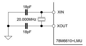
Figure 6. Crystal Connections
