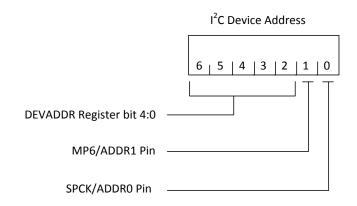
Figure 35. I<sup>2</sup>C Device Address
