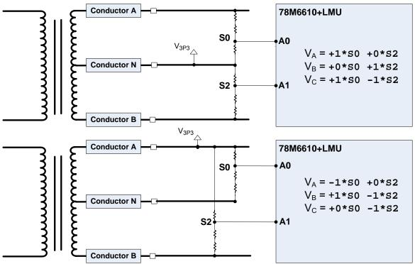
Figure 11. Example Voltage Configurations
