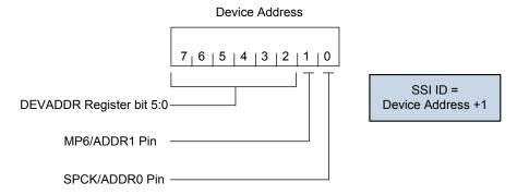
Figure 28. Device Address Configuration
