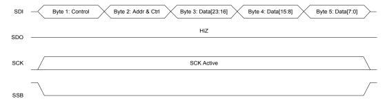
Figure 32. SPI Timing Continuous Clock
