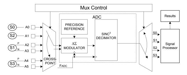
Figure 8. AFE Input Multiplexer
