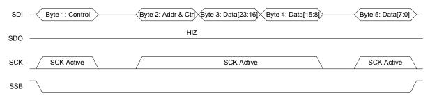
Figure 33. SPI Timing Gapped Clock
